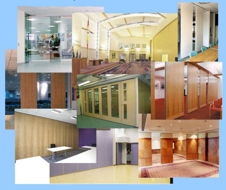
Operable walls provide custom built top hung partitions with a wide range of layout, stacking and finish options. Pass doors can be incorporated into panels or be full height at one or both ends. Glazed & semi-automatic options are available
